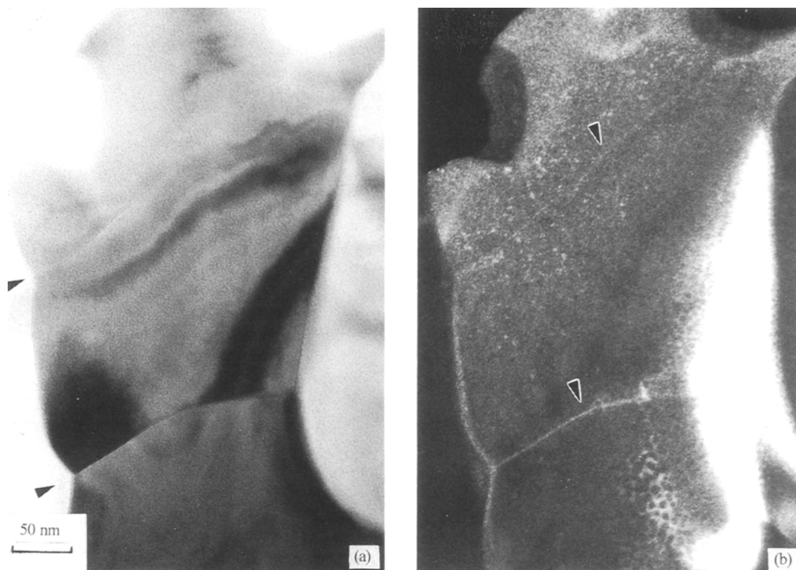
Figure 7 (a) Bright-field and (b) diffuse dark-field micrographs demonstrating the multigrain second-phase pockets present in the material with 10 vol % additives, after a post-sintering heat treatment. The “bumps” on the \text{Si}_3\text{N}_4 grains at the second-phase grain boundary are arrowed in (a), and the thin amorphous layer between the \text{Si}_3\text{N}_4 and secondary phase grains, and between the two secondary phase grains can be seen in (b).
